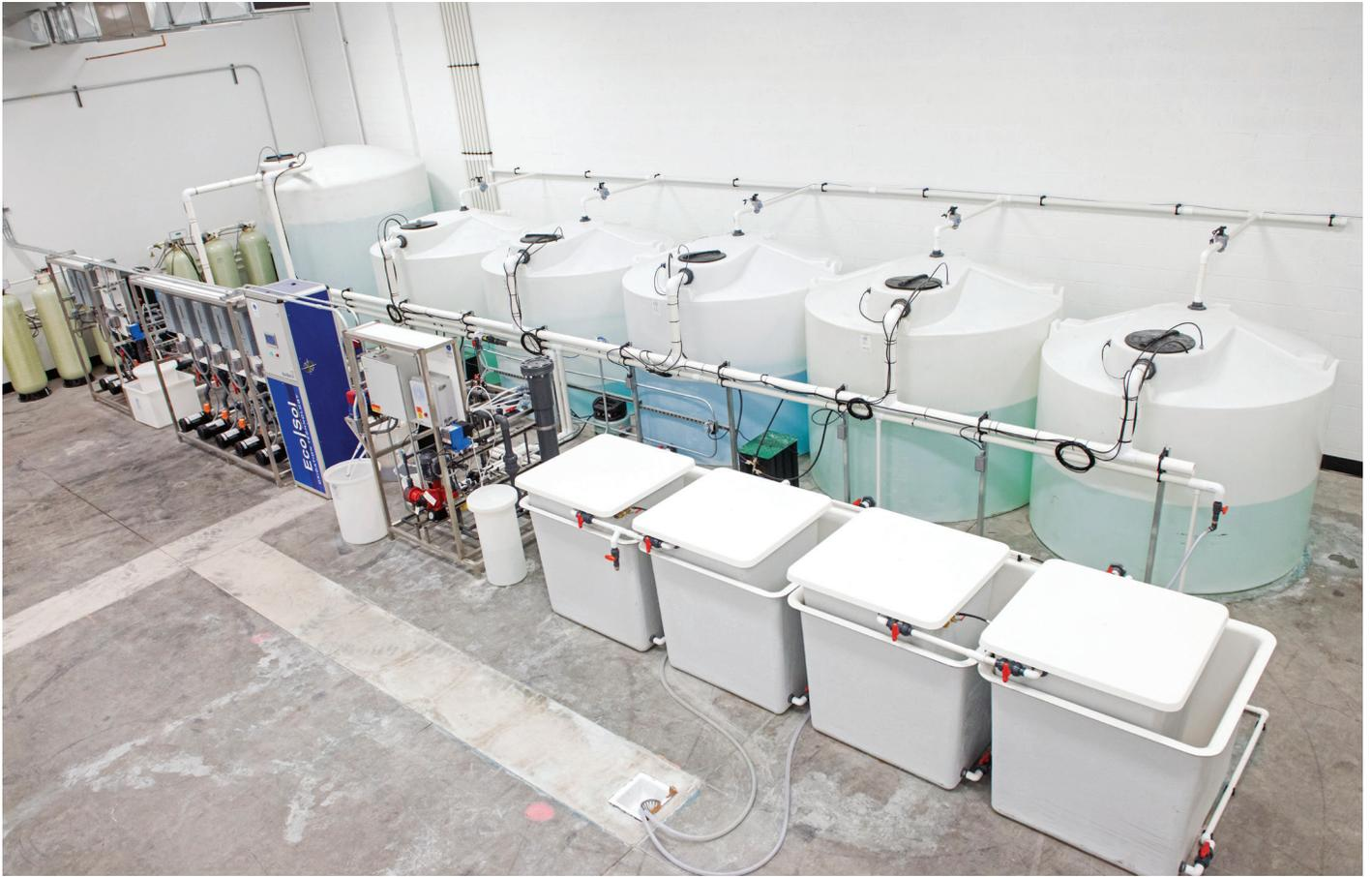
Plants are automatically watered and fed via this fertigation room at Green Thumb Industries. If levels are not perfect, the cultivation team can adjust them using mobile devices.
